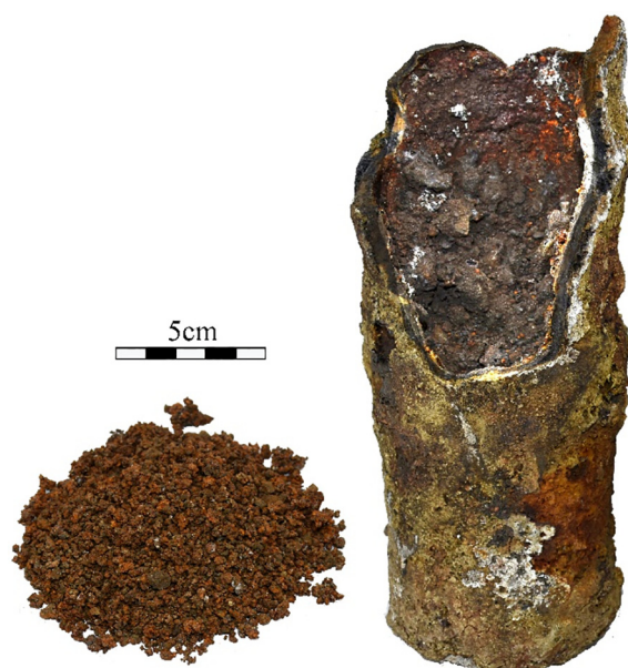
Fig. 9. The granular slag tipped out from the pots (left) and the slags attached inside the pot TP4 (right).
