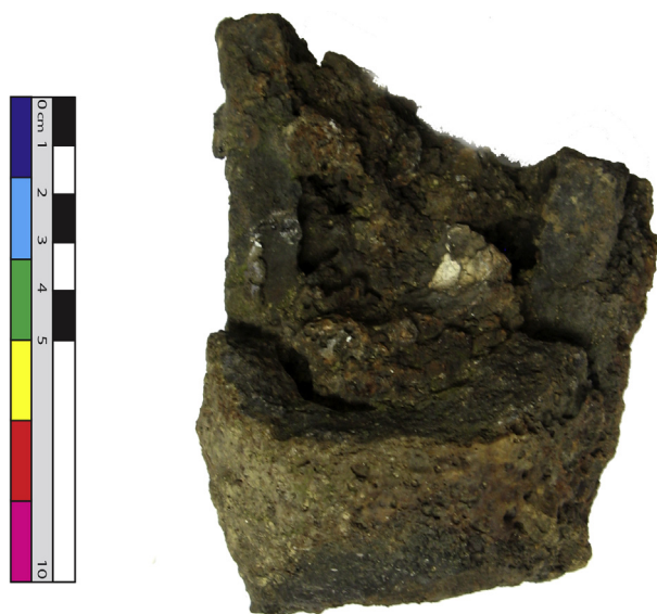
Fig. 5. Rusty slag with white inclusions within the ceramic pot in SDB7.
