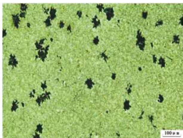
Figure 10: The microstructure of a malleable iron tool excavated from Chengcun, Fujian province.
