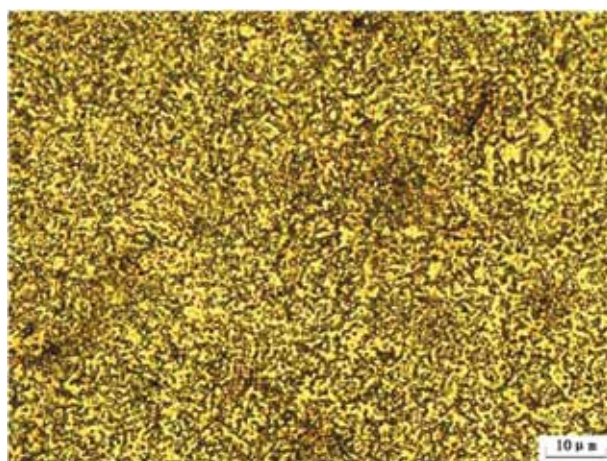
Figure 11: The microstructure of decarburised steel objects excavated from Hezhang, Guizhou province.
