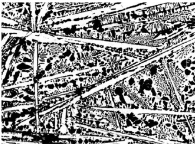
Figure 1: The microstructure of the earliest known cast iron fragment dating to the 9 th -8 th century BC and found at the Tian-ma Qucun sites in Shanxi Province.
