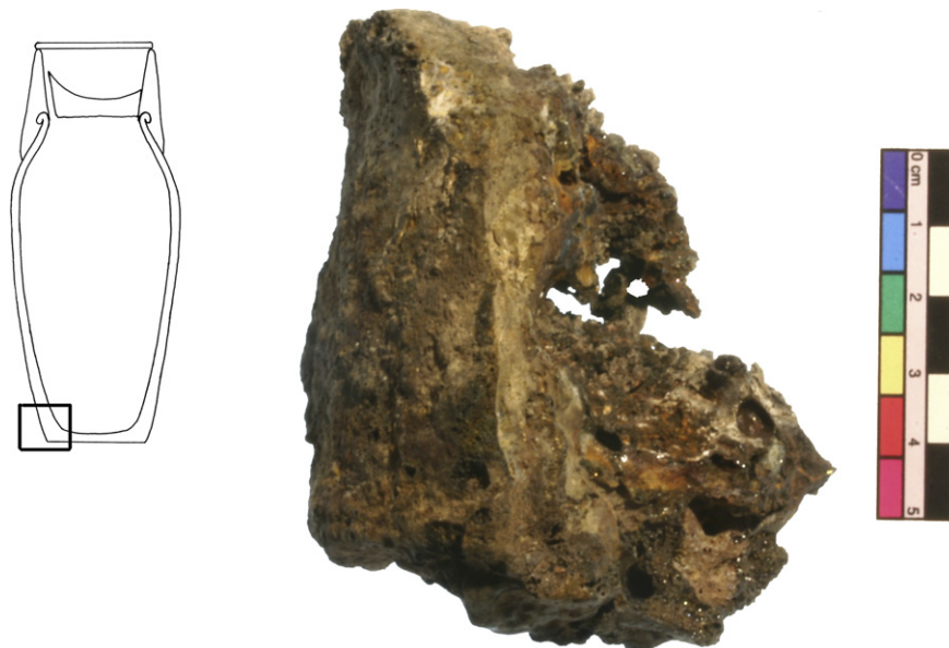
Fig. 13. Slag adhering to the bottom of pot YMB1.
