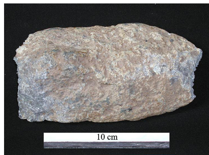
Fig. 4. One of the zinc ingots discovered at Miaobeihou in the 1980s.
