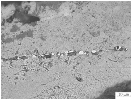
Figure 4 Laminated two-phase slag inclusions of M27: 91 (unetched).
