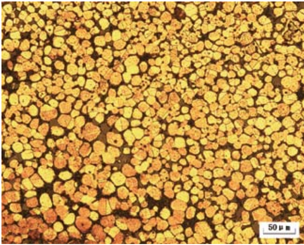
Figure 7 Sample ZGM36-2 microstructure, etched, equi-axed and twinned grain with intergranular lead prills and sulphide inclusions.
