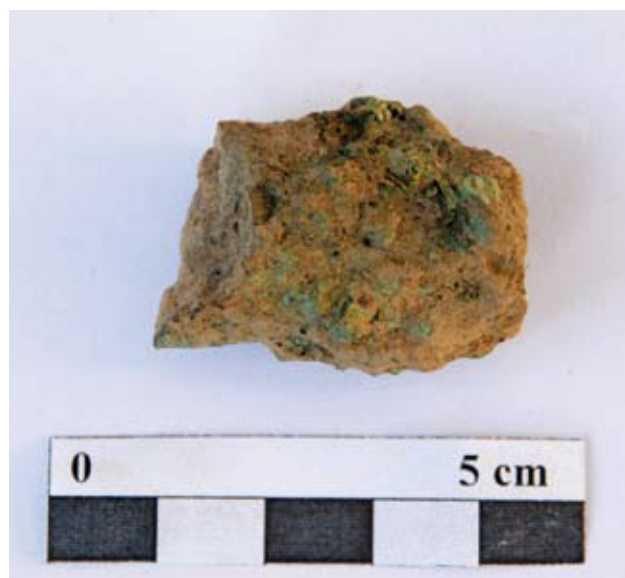
Figure 16 Vitrified ceramic casting cores from Zhaojiatai.
